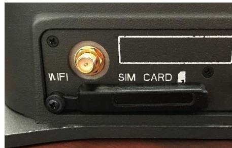
Figure 2-14 Secure the SIM Card Cover
