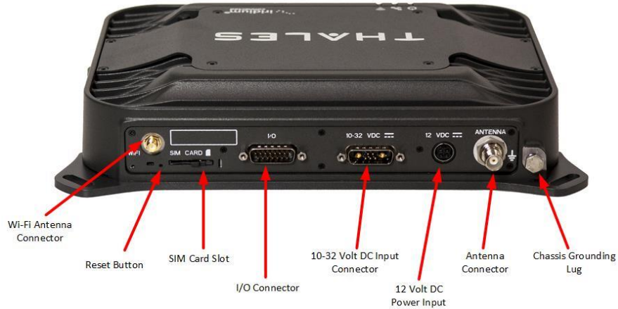
Figure 1-5 Below Deck Unit (BDU) Back Panel Detail
